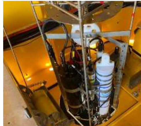
Weather station and SilCam on the buoy
