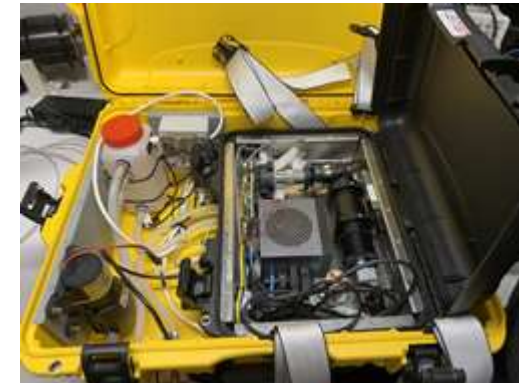
Microplastic sensor testing on the buoy
